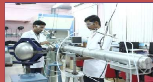
Single Pulse Shock Tube (For combustion studies)
