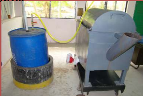
Applied Microbiology Biogas collection from Jatropa oil seed cakes
