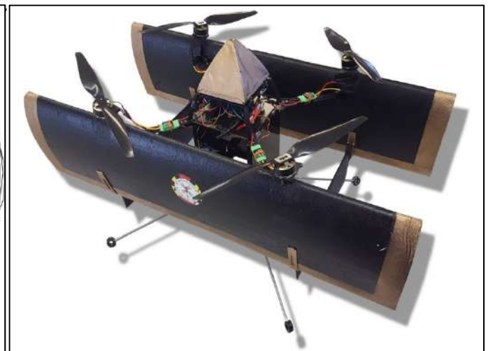
Quad-Rotor Bi-Plane Tail-sitter configuration for efficient VTOL/forward flight
