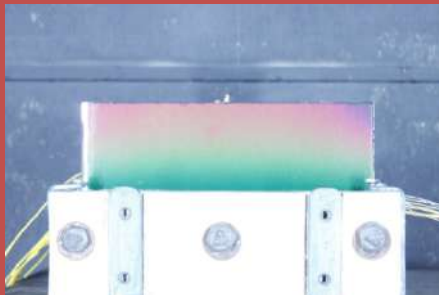
Temperature field with thermo chromic liquid crystals
