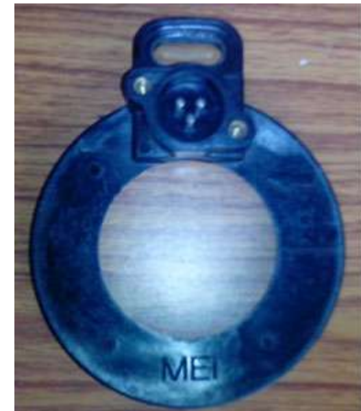
Brake wear sensor for heavy vehicles
