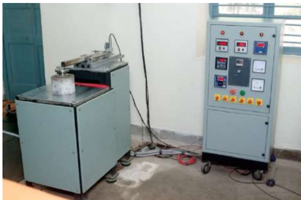
Sliding wear test (Pin-on-Disc)
