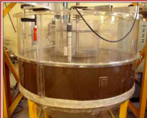
Annular flume (to study about sediments)
