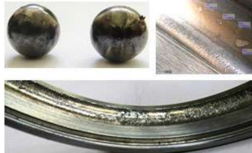
Failed bearings samples after dismantling
