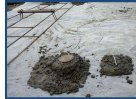
Field Instrumentation to Evaluate Load & Warping Stresses Back to Top
