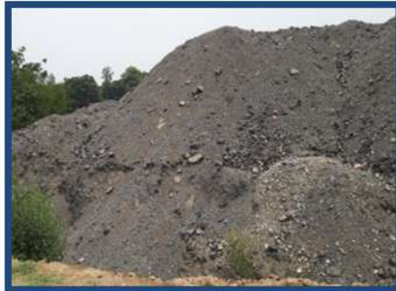
Pavement Demolition Waste
