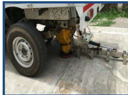
Pavement Structural Evaluation via FWD
