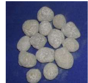
Sintered & cold-bonded fly ash aggregates
